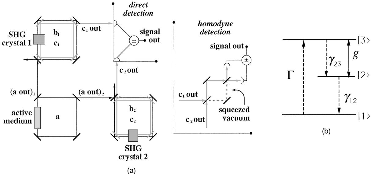
Fig. 2. (a) Schematic representation of the system analyzed, showing two detection methods. The spectra obtained by the two methods are equivalent. (b) Energy-level scheme of the laser atoms.
