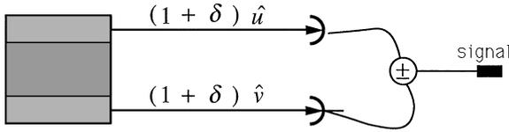
Fig. 1. Schematic representation of a system that emits beams with independent quantum noise and correlated classical noise.
