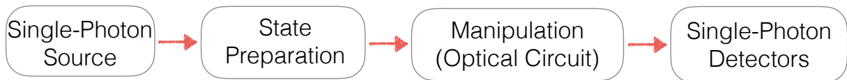
Figure 2.2: General structure of photonics experiments. We start with a single-photon source like SPDC or quantum dots. If we do not obtain the desired state from the source, we then enter a preparation stage of the desired state. For instance, if one obtains horizontally polarized photons from the source and one wishes a superposition of horizontal (H) and vertical (V) polarizations photons, let the photon pass through a 22.5^\circ Half-Wave Plate (HWP) followed by a Polarization Beamsplitter (PBS). This will make a qubit as well. Next, the manipulation stage encapsulates the particular application, for example, a quantum controlled-not gate, or a quantum simulation experiment. Finally, we must detect the photons.
